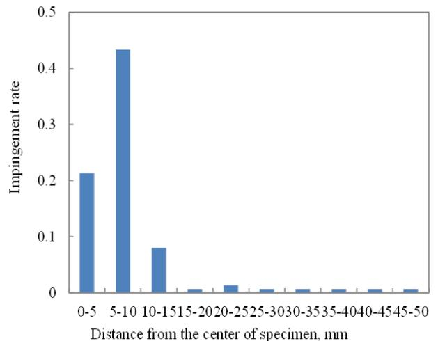
Figure 13. Histogram of impact location of particles
