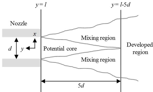
Figure 6. The structure of turbulent jet flow
