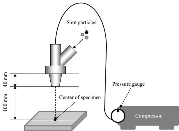
Figure 1. Experimental setup for shot peening process
