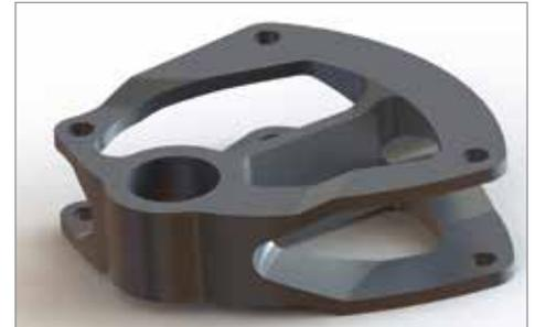
*CAD model of the optimized rocker design.*
