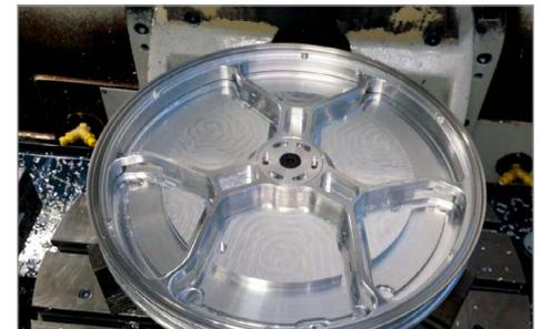
Wheel rim in the milling manufacturing step.
