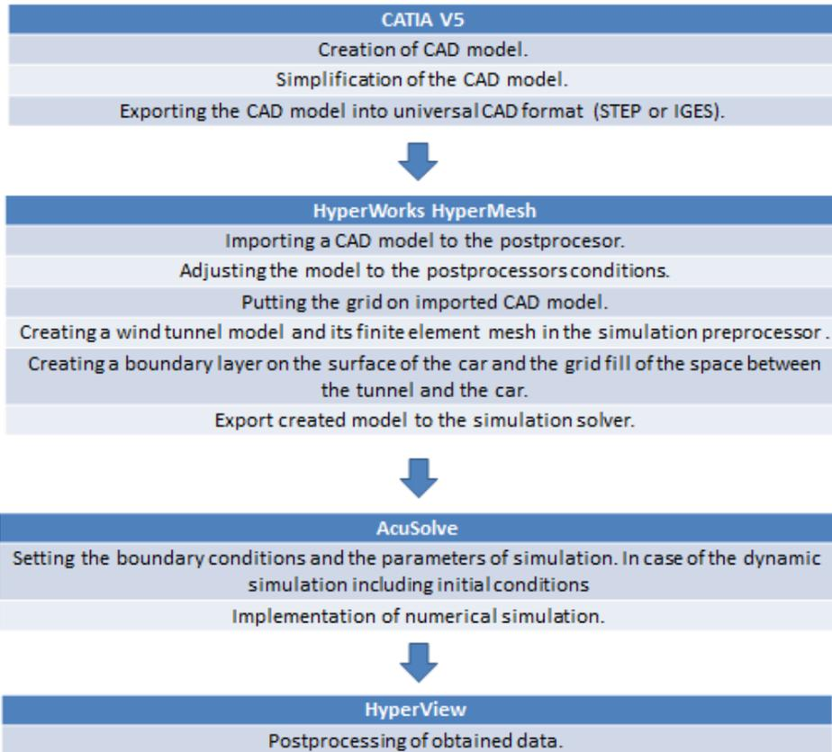
Fig. 1. Diagram showing the developed methodology of the research
