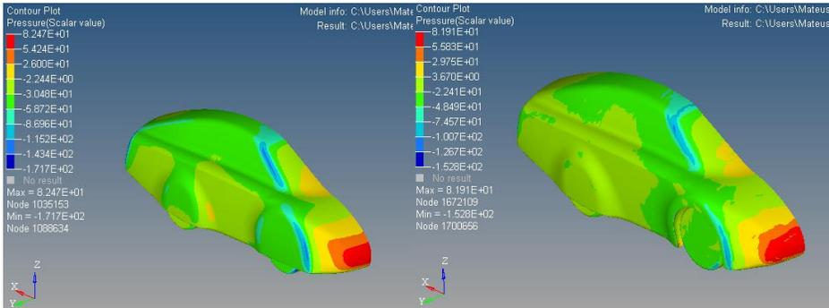
Fig. 3. Comparison of air pressure distribution on the surfaces of development versions v3 (pictured left) and v4 (pictured right)
