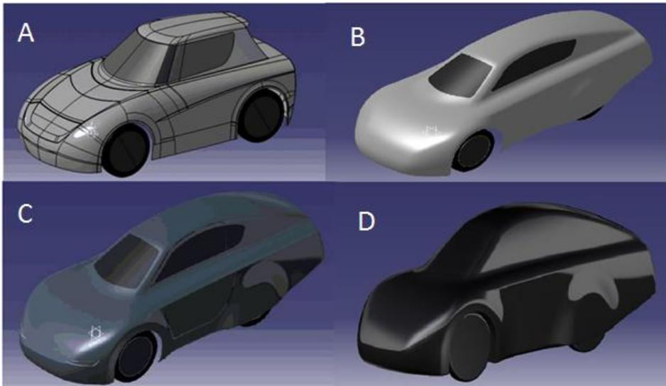
Fig. 2. CAD models of the urban car Bytel in the development versions a) v1 b) v2 c) v3 d) v4<sup>1</sup>
