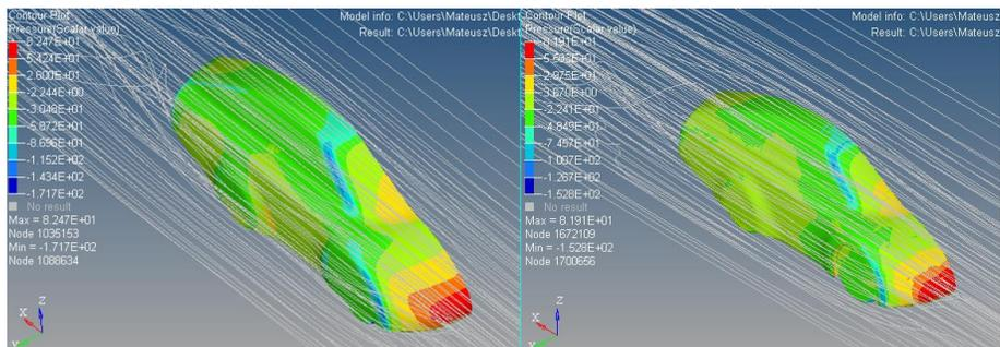
Fig. 5. A comparison of air streams amounting car. Development version v3 (pictured left) and v4 (pictured right)
