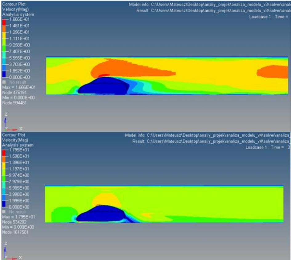
Fig. 4. Comparison of air velocity distribution in the plane coinciding with the plane of symmetry of the car. Development version v3 (pictured top) and v4 (pictured below)
