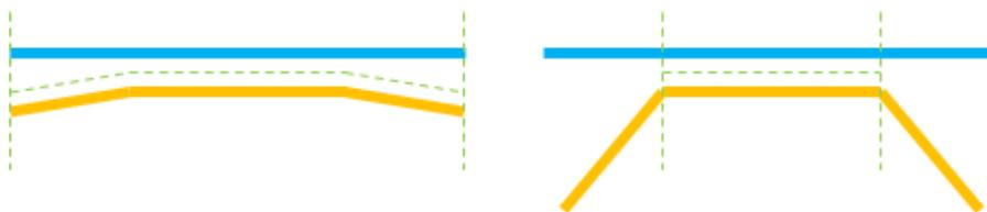
In these examples, the dotted green lines indicate the area where imprint will take place when using a **feature angle** of 30 degrees.
