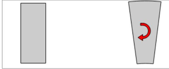
Figure: A small section of the beam before and after bending moment is applied
